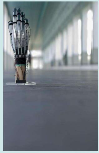
The glove is able to generate up to 40 Newton's of holding force on each finger with just 200 Volts and only a few kilowatts of power.
