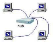
**ADVANTAGES:** centralized monitoring, failures do not affect others unless it is the hub, easy to modify.
