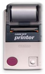
The system will print a test message reading "Hello" if it is turned on while the feed button is held. According to the manual, this is used to test if the printer functioning properly. To get around using six AA batteries (1.5 volts each) for the printer, a single 9V battery can be used if wired properly, because the printer requires 9V DC.A roll of the American Game Boy Printer paper came in red, blue, yellow and white, with an adhesive backing. It had a width of 38mm and a diameter of
