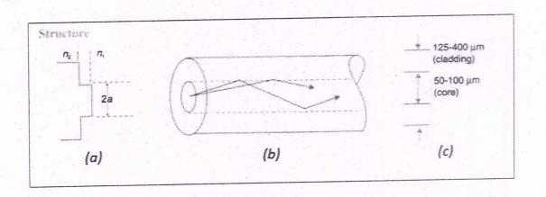
The figure shows (a) its R.I. profile, (b) Ray paths (c) typical dimensions.
