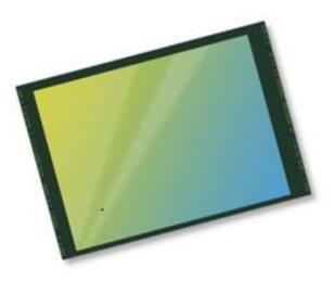
The unique 16-cell binning of the OVB0B delivers 4K2K video quality in 12.5MP mode with 2.44  $\mu$ m-equivalent pixel size using near pixel 4×4 binning, especially in
