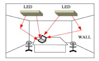
Optical wireless communications (OWC) is a form of optical communication in which unguided visible, infrared (IR), or ultraviolet (UV) light is used to carry a signal. OWC systems operating in the visible band (390–750 nm) are commonly referred to as visible light communication (VLC). VLC systems take advantage of light emitting diodes (LEDs) which can be pulsed at very high speeds without noticeable effect on the lighting output and human eye.
