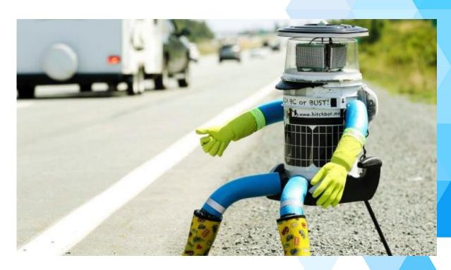
On the inside, hitchBOT is a bit more high-tech. The robot is equipped with a GPS system so researchers can track its location. It also has a built-in camera that snaps a few pictures every 20 minutes to document the bot's travels. The robot can post the data it collects about its travels to social media sites, such as Twitter, Facebook and Instagram.
