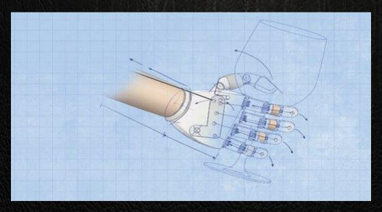
How It Works: The Stark Hand: The prosthetic hand attaches to a cable that runs from a shoulder harness worn by an amputee. A lever on the palm opens all five fingers at once, and separate cables in
